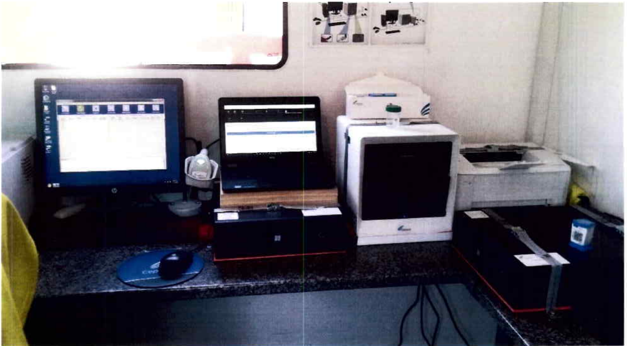
Image 8. Gene Xpert equipment procured through UNDP on one of the leased mobile trucks used to process sputum samples
