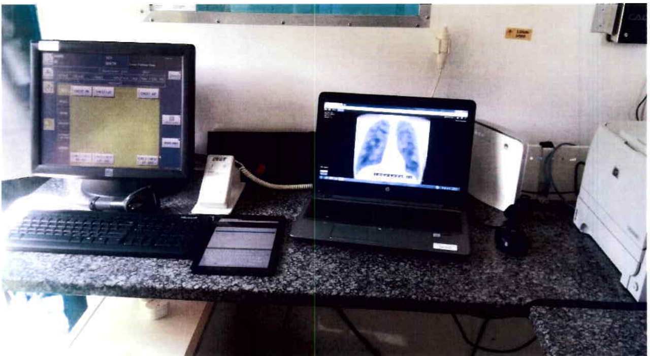
Image 9. Chest x-ray image processing monitor (left) and a Chest X-ray image (right) processed through the CAD4TB software displaying a heatwave of the lung area. Equipment and software procured by UNDP.
